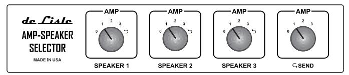
The four switches on the front panel route the corresponding speaker to the selected amplifier. For example, if the "Speaker 1" knob is set to the "2" position, the cabinet connected to the "Speaker 1" jack on the rear panel will be routed to the amplifier connected to the "Amplifier 2" jack. If two cabinets are routed to the same amplifier, they will be connected in parallel. Set the knob to the "0" position if you do not want to connect that particular cabinet to an amplifier.
